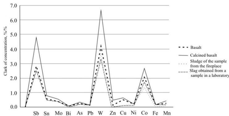
Figure 6. Geochemical spectra of clarks of chemical concentrations elements in the rock samples from the mound of the Altynshoky hill. From top to bottom: metabasalt, calcined metabasalt, slag sample from the mound, slag received from basalt sample in the laboratory
