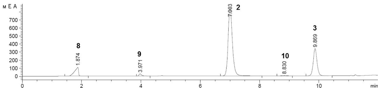
Figure 1. HPLC of DMGU hydrolysis in 1 day
