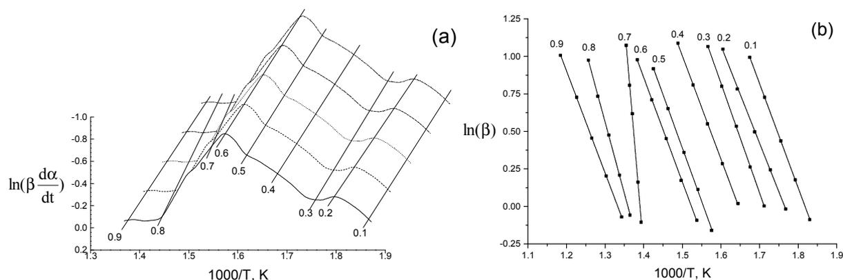
Figure 3. Graphical results of analysis determined by the methods of Friedman (a), Flynn-Ozawa-Wall (b) for CO<sub>2</sub>-extract distilled from *Scabiosa ochroleuca* (cream scabious) at heating rates from 5 to 25 deg/min
