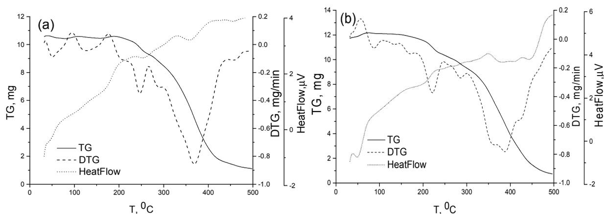
Figure 1. TG, DTG/HF curves for CO<sub>2</sub>-extracts: *Scabiosa ochroleuca* (a), *Scabiosa isetensis* (b) in air
