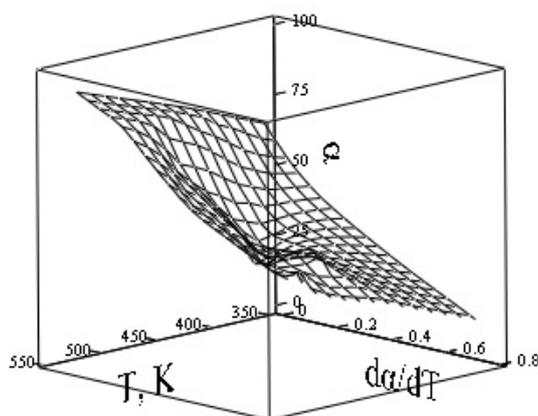
Figure 4. Surface of  $\text{CO}_2$ -extract distilled from *Scabiosa ochroleuca* in three-dimensional space: dependence of reaction rate ( $d\alpha/dT$ ) from temperature ( $T$ ) and conversion degree ( $\alpha$ ) in air
