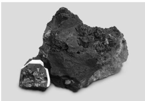
Figure 3. Slag in a crucible and a historical sample
