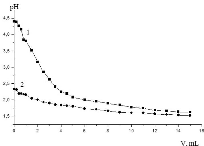
1 — a curve of potentiometric titration in absence of a metal ion;
