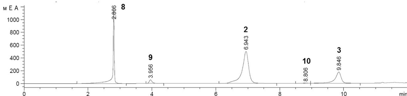
Figure 2. HPLC of DMGU hydrolysis in 3 days
