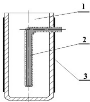
1 — glass cup; 2 — internal electrode; 3 — external electrode
