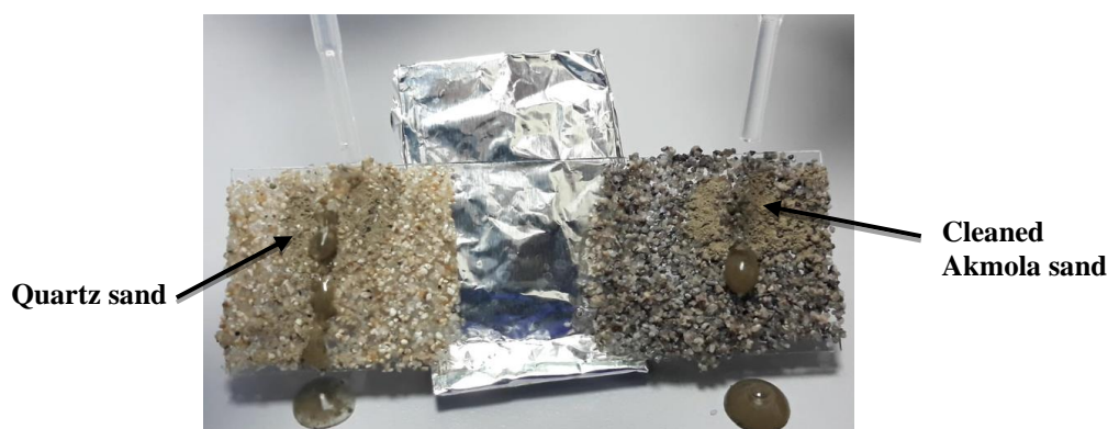
Figure 11. Self-cleaning properties of superhydrophobic surfaces of quartz and Akmola region sand
