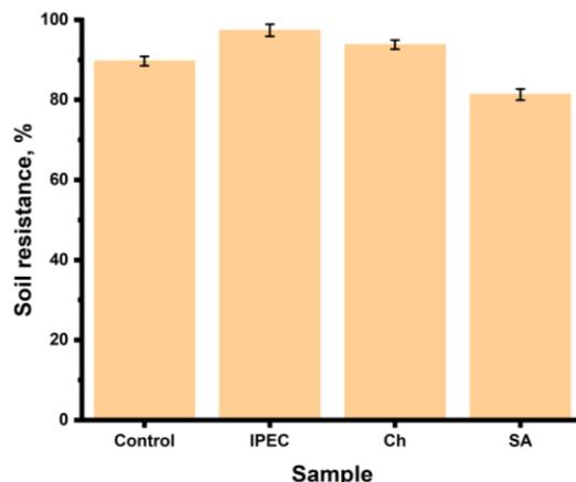
Figure 5 Diagram of soil resistance to trickle erosion
