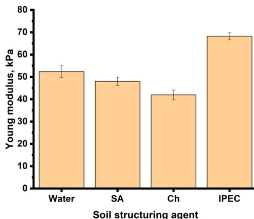
Figure 3. Mechanical properties of soil structurates
