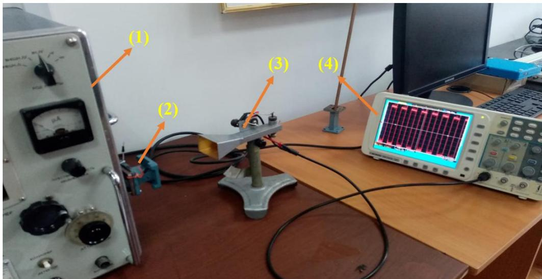
1 — microwave generator; 2 — waveguide instrument (IEC Standard R100, X Band);
