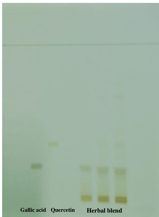
Figure 1. Developed HPTLC plate under UV light at 254 nm
