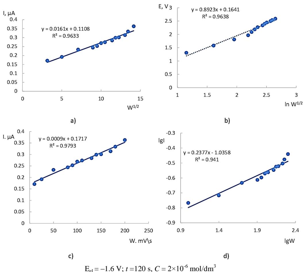
Figure 2. Dependence of the methionine oxidation current on the square root of the potential sweep rate (a), the dependence of the potential on  $\ln W^{1/2}$  (b), the dependences of the current on the potential sweep rate (c) and  $\lg I$  on  $\lg W$  (d)
