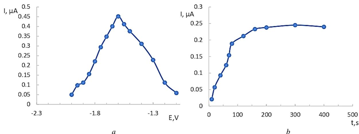
Figure 4. Dependence of the methionine electrooxidation current on the accumulation potential at the modified electrode ( $t = 120$  s,  $W = 80$  mV/s,  $C = 5 \times 10^{-6}$  mol/dm<sup>3</sup>) (a) and the dependence of the methionine electrooxidation current on the accumulation time ( $E_{cl} = -1.6$  V,  $W = 80$  mV/s,  $C = 2 \times 10^{-6}$  mol/dm<sup>3</sup>) (b)
