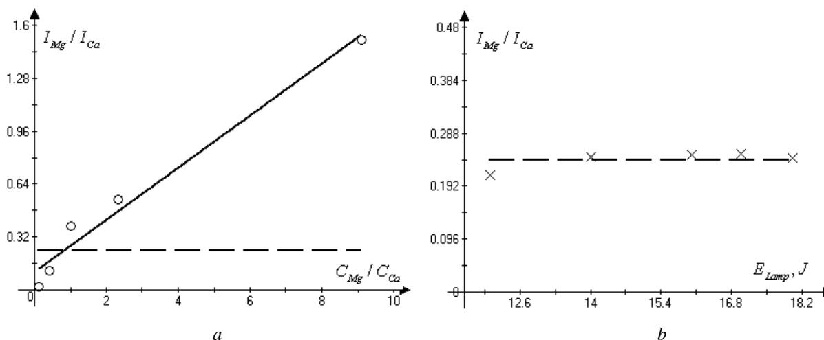
Figure 5. Dependence of the ratio of the intensities of the Mg(I)<sub>293,67</sub> and Ca(II)<sub>315,9</sub> lines on the: a) ratio of the concentrations of elements; b) the energy of the laser pump lamp
