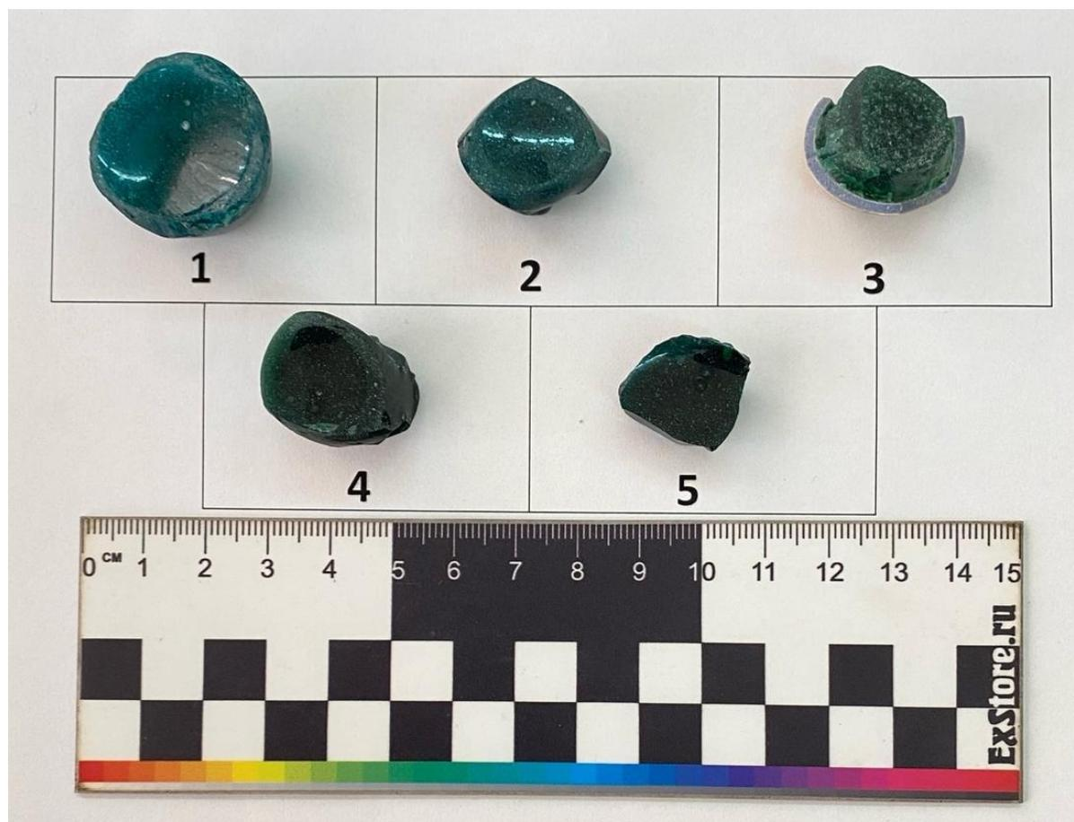
Figure 2. Calibration samples of enamel
