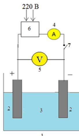
1 — electrolyzer; 2 — titanium electrodes; 3 — electrolyte (different medium);
