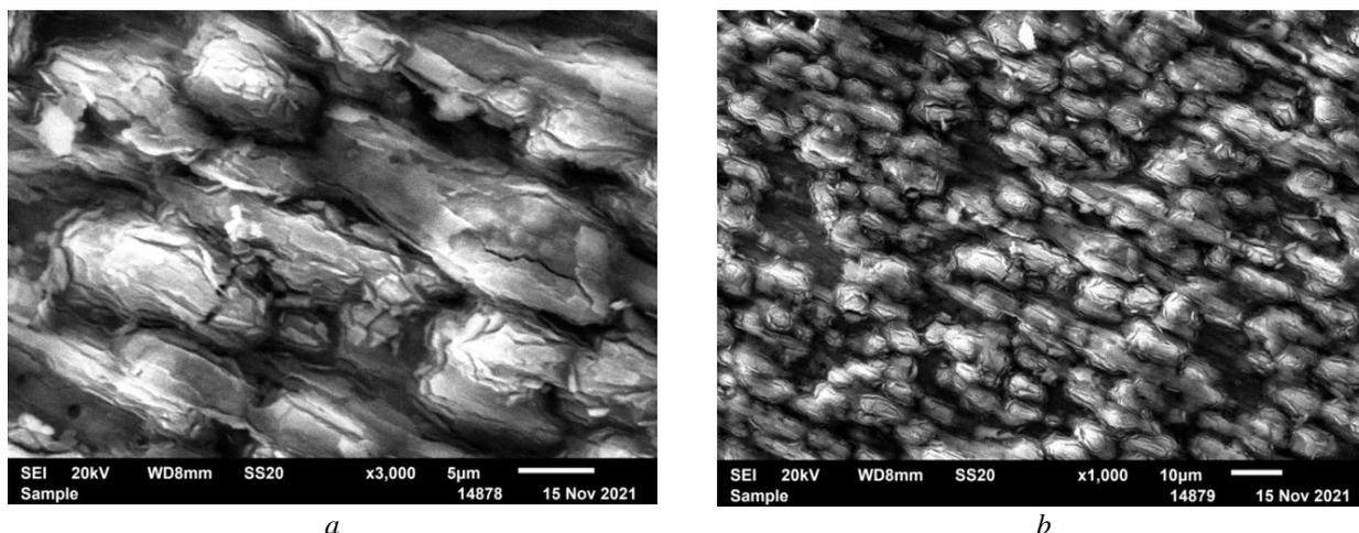
Figure 5. Micrographs of titanium dioxide films produced on the surface of a titanium anode in a sulfuric acid solution with an increase: a) 3000 times; b) 1000 times
