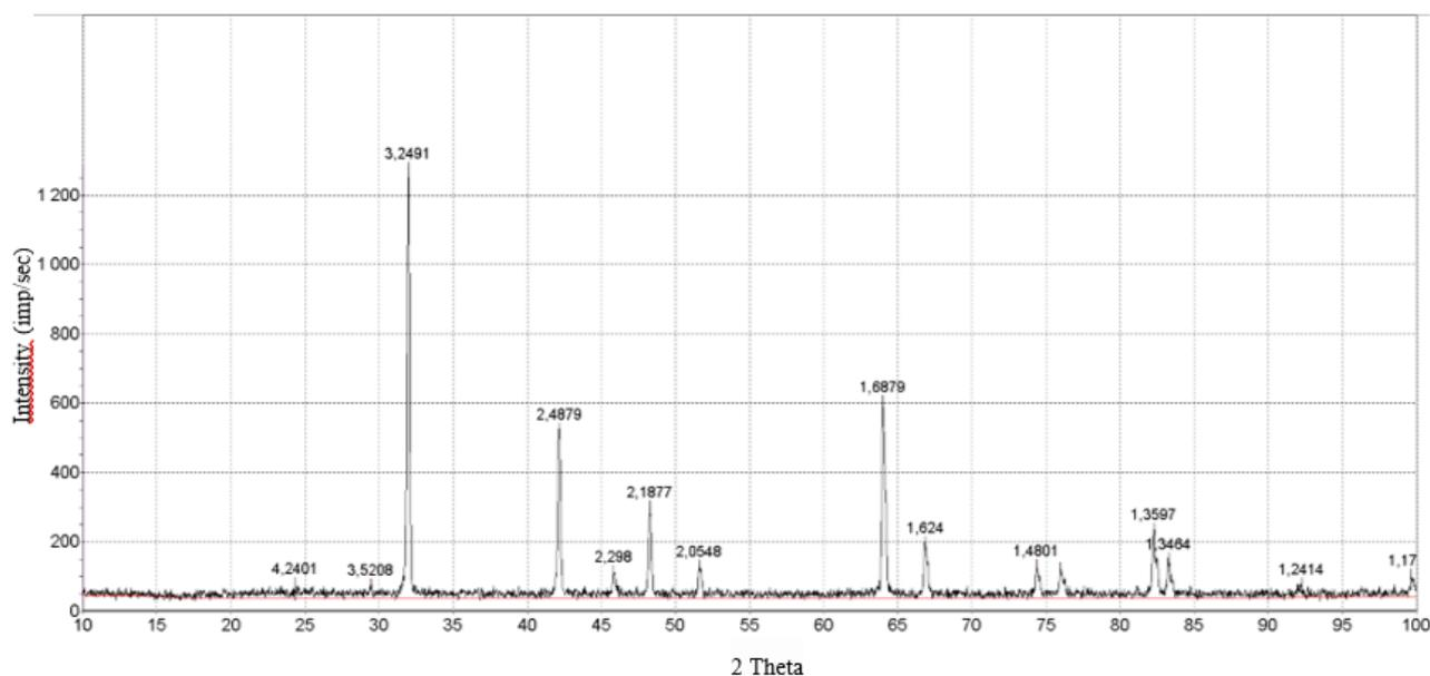
Initial angle = 10,00; Final angle = 100,00; Step = 0,020; Expos. = 0,6; Rate = 2g/min; Max. number of impulses = 769;
