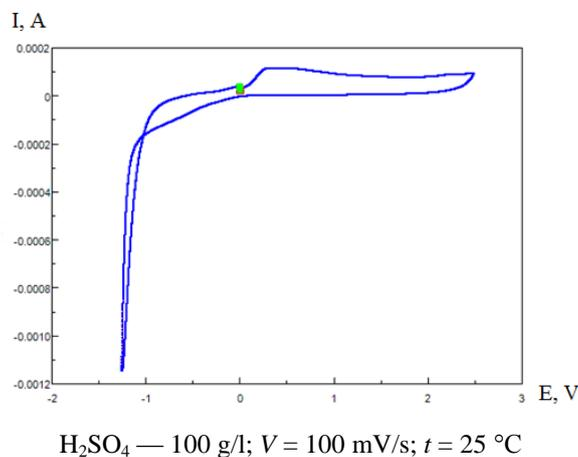
Figure 2. Cyclic anode-cathode voltammograms of titanium electrode in sulfuric acid solution
