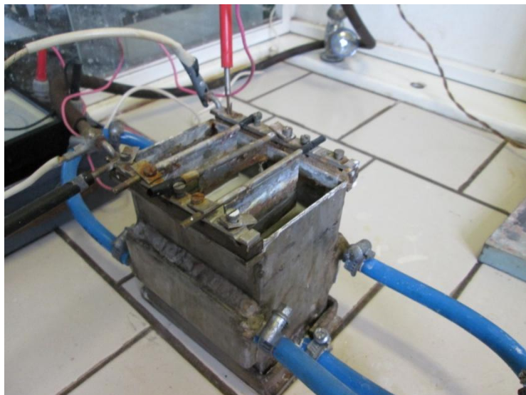
Figure 3. Water-cooled electrolyzer for laboratory extraction of gallium from alkaline-aluminate solutions
