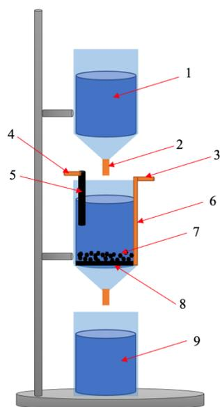
1 — Pb (II) containing wastewater sample; 2 — water flow controller;
