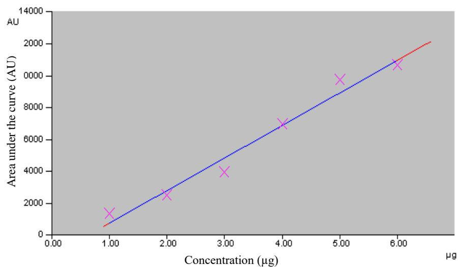
Figure 4. Linearity of berberine standard (1 µg/band – 6 µg/band)
