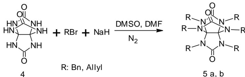
Figure 2. A synthetic protocol for alkyl derivatives of 3,7,10-trioxo-2,4,6,8,9,11-hexaaza[3.3.3]propellane
